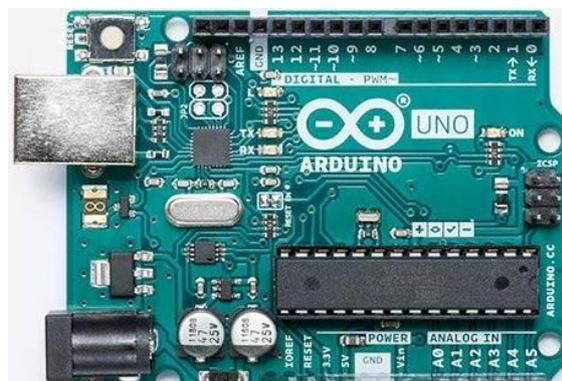
**Gambar 2.5** Microcontroller Microchip ATmega328P
