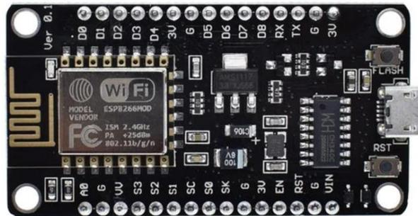
**Gambar 2.4** Board NodeMcu
